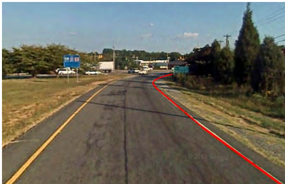
Image from Google Earth shows gore striping, stop line placement, and sweeping curve for right turns at US 421 Off-Ramp.
