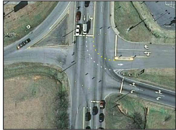
Rendering showing application of (1) white and yellow dotted line pavement markings to delineate movement from southbound US 601 onto Pine Street and (2) through arrow on Pine Street departure leg.
