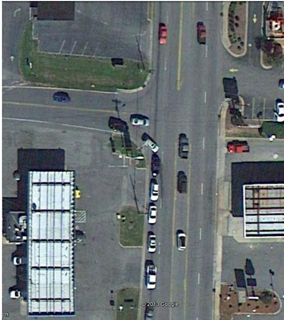
Image from Google Earth showing left-turning and right-turning vehicles side-by-side on Beroth Drive at US 601.
