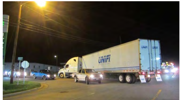
Photos showing the difficulty faced by a left-turning tractor trailer in completing its maneuver from northbound US 601 onto Beroth Drive. A number of other vehicles were also impacted; e.g., the SB vehicles whose path was blocked were forced to come to a complete stop, and the pickup truck desiring to turn left from Beroth Drive ultimately turned right to give the truck the space it needed.
