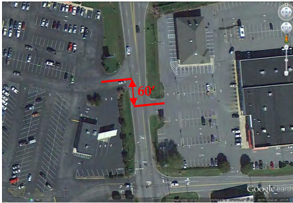
Aerial image from Google Earth showing offset between CVS and unsignalized Colonial Shoppes driveways along US 601.
