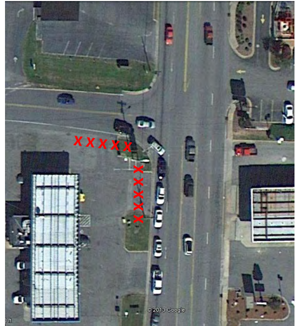
Consider closing northern BP driveway along US 601 and installing a raised curb/island to better control vehicular movements.
